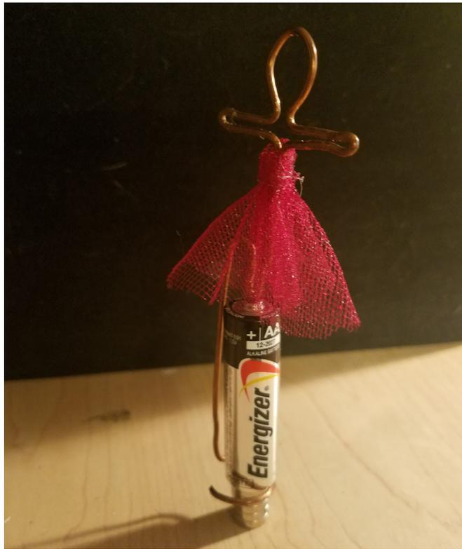
Using a battery and some magnets, create a spinning motor and explore electromagnetic principles!
